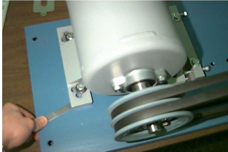
Soft-Foot Check Using Feeler Gages
