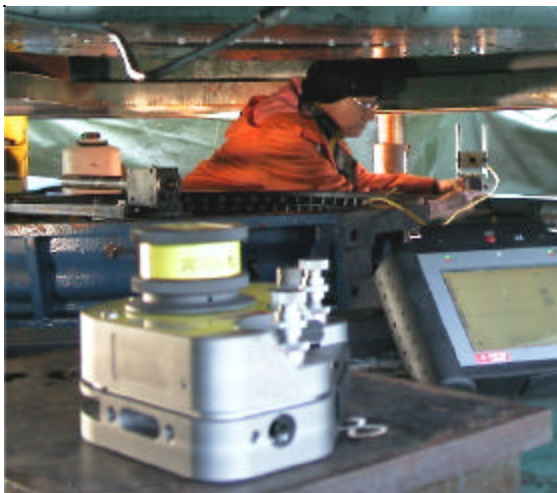
The laser transmitter sweeps a flat plane.
